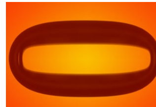
spinning drop inside capillary
