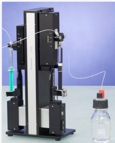
The LDU 25 liquid dosing unit can vary concentrations automatically.
